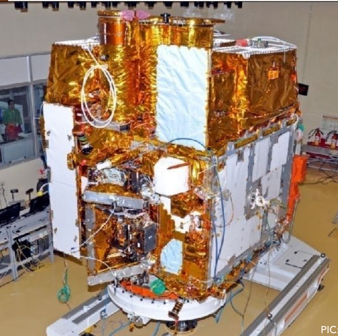
Integrated AstroSat before launch weight: 1.5 ton
